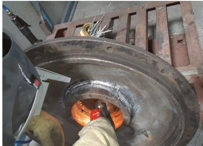
PHOTO- C (Preheating & Gouging)
