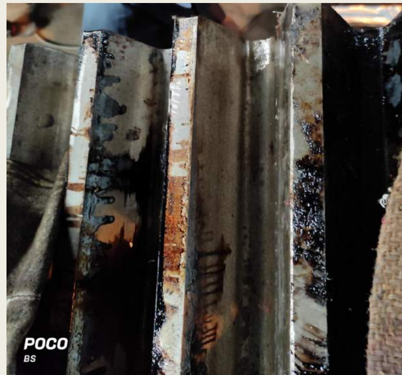
Photo:03 - Cracked area of the Gear
