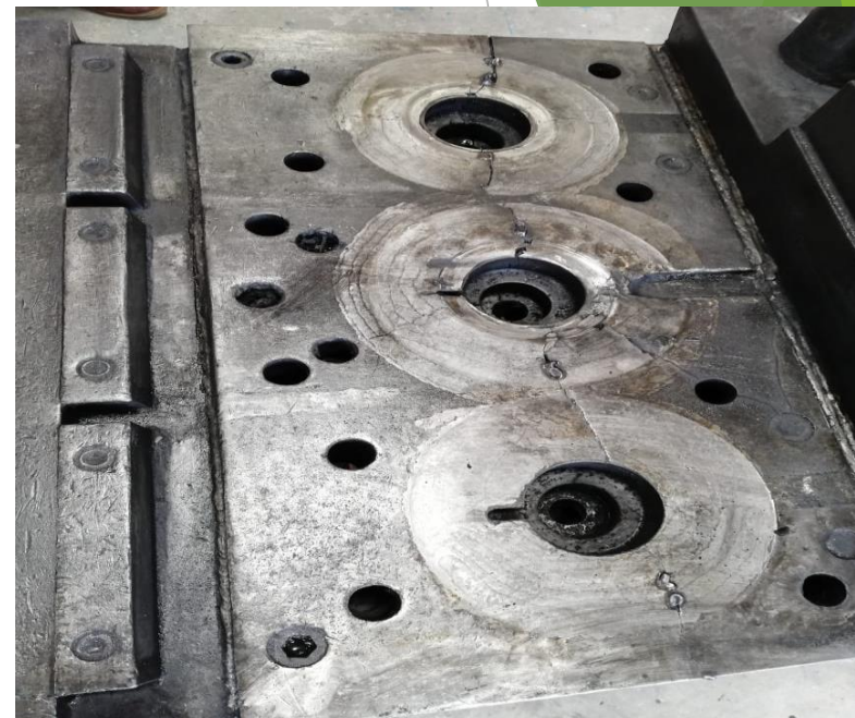
Photo:03 - Bolster for Repair
