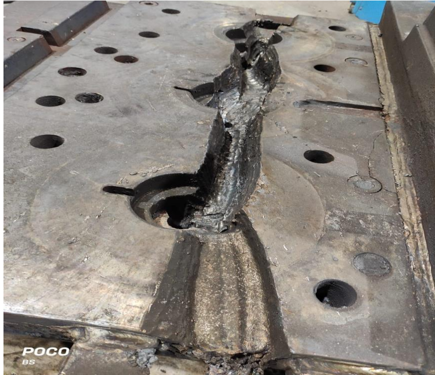
Photo:05 - Removed the crack by Gouging process & Grinding
